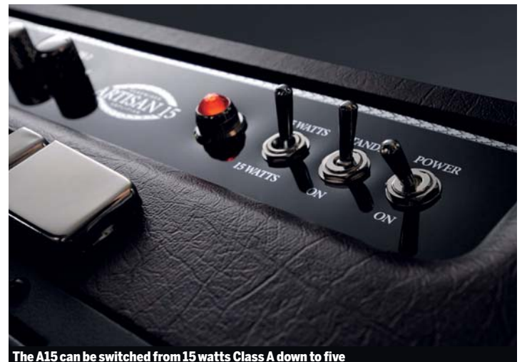
The A15 can be switched from 15 watts Class A down to five
